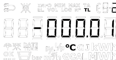
Figure 18 - Setting up negative TL2 in SETUP loop, the - will be flashing when on the sign position and stays on when moving to another decimal.
